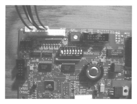
In this example switch 1 is off all others are on. The numbering scheme is binary so if the desired address is 2 then switch 2 is off all others on. Address 3 would be switches 1 and 2 are off all others on. See attached chart for all address 1 thru 96. The first 10 are shown here.
